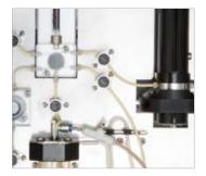
From the oil-free air compressor to the special teat cleaning cup and food grade stainless steel milk transfer lines – milk quality is prioritised in the DeLaval VMS. Four optical, quarter milk meters monitor deviations and abnormalities in flow rates, yields, conductivity and blood levels. Abnormal milk can automatically be diverted away from the main tank. Meanwhile the management software records all the data and events to facilitate your management decisions.
